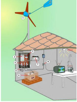
Figure 3: The components of a small wind energy system.
